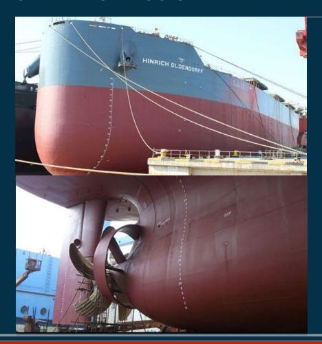
The spoon bow of our new Newcastlemax bulk carriers is designed to optimize the flow of water around the bow and provide optimal cargo on draft characteristics.
